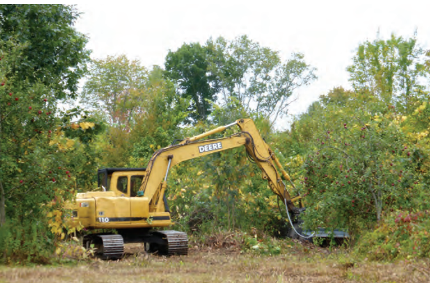
High-speed forestry mulching head on a tracked machine can reduce non-native invasives so that more-desirable plants can compete. Credit: Richard Martin
