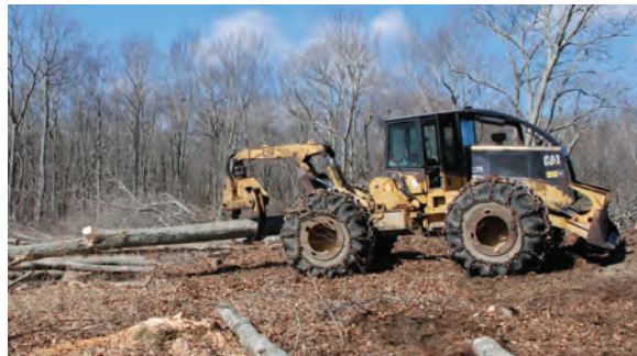
This grapple skidder can quickly and efficiently create large patches of young forest. Credit: Judy Wilson
