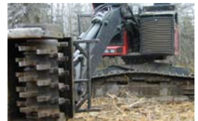
In some situations, mechanical cutting of alder can be an efficient and economical practice. A brontosaurus has a specially adapted cutting head./Scot J. Williamson
